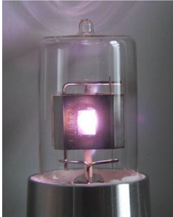
A DEUTERIUM ARC LAMP, which is continuous over the ultraviolet region (190–400 nm)
