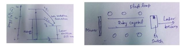
The design of Ruy laser is made up of a ruby crystal rod with a flash lamp around and they are arranged in a reflection cavity. At one end, a mirror is placed to reflect the pulse. At the other end a Q switch is used either to allow the laser to pass or to reflect it back through the cavity for another cycle.
